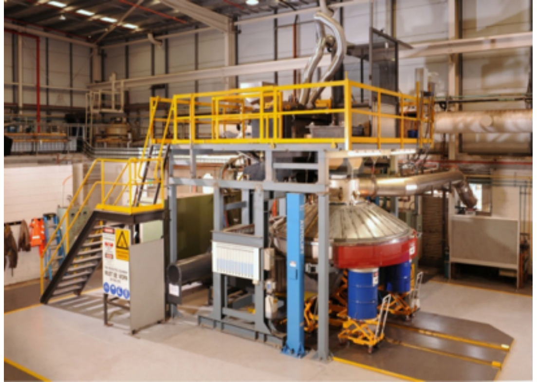
Semi-industrial scale DSG pilot plant ( \phi 3 m & 100 kg/min).
