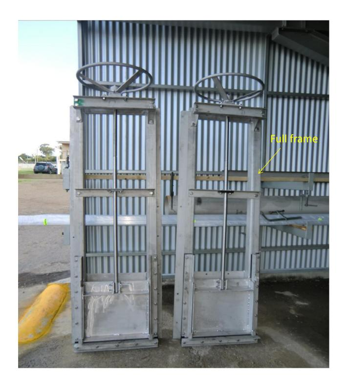
Ready to leave the workshop after cycle testing Thrust tube type
